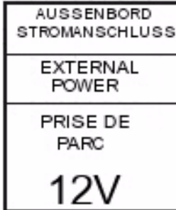
Figure 2-7 If installed, at the access door to the external power receptacle behind the wing on the aircraft's right side.
