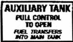
Figure 2-9 If optional extended range fuel tank is installed, placard must be placed near to the fuel transfer control.
