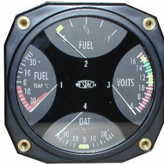
Example of the Westach quad indicator installed on model #3
