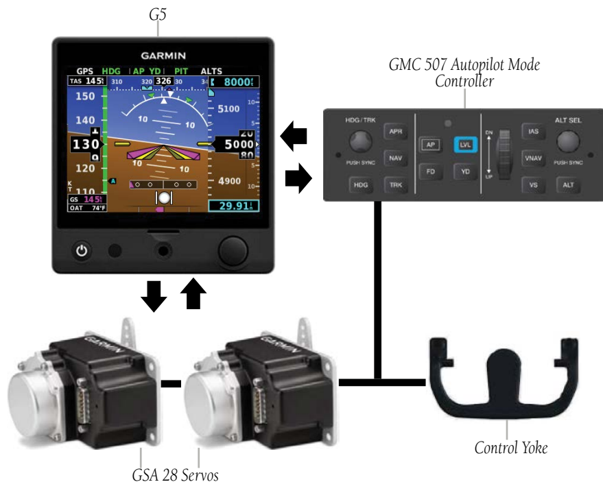
Figure 3-2 Core GFC 500 System
