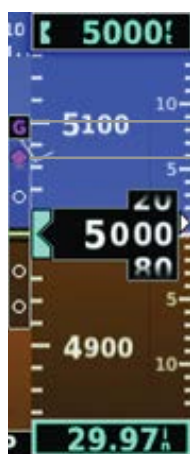
Figure 2-26 Vertical Deviation Indicator (Glidepath GPS Source) - PFD
