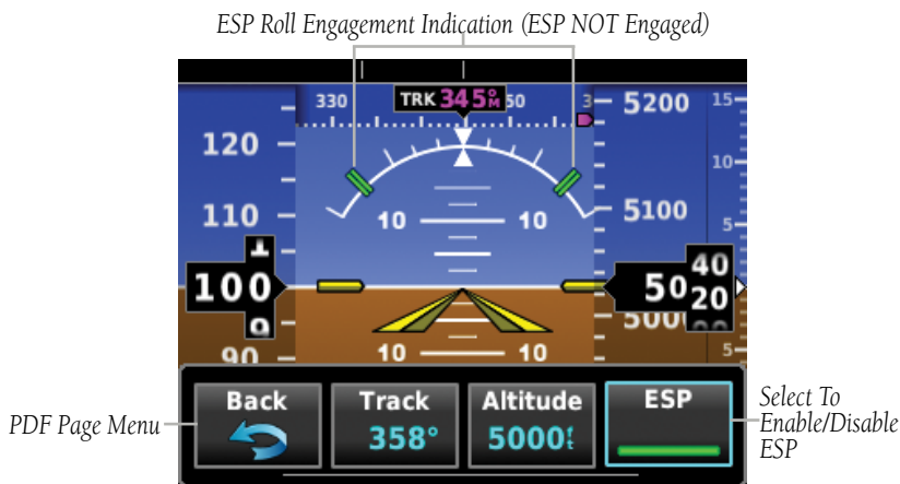
Figure 3-26 AFCS (ESP Enabled)
