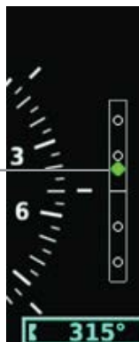
Figure 2-25 Vertical Deviation Indicator (Glideslope ILS Source) - HSI
