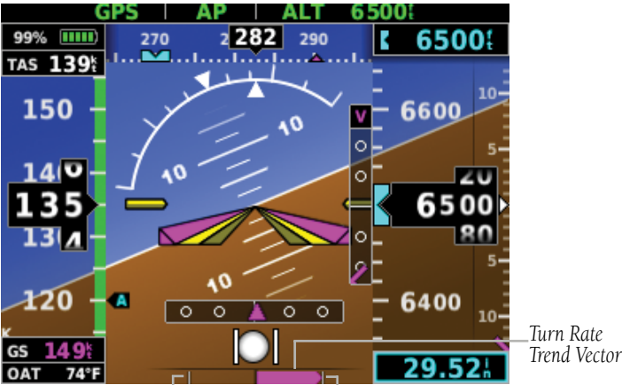
Turn Rate Indicator (Standard Rate Tick Marks)
