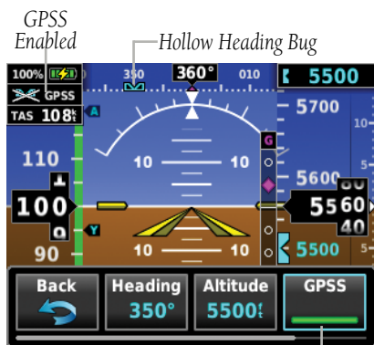
Figure 4-3 GPSS Enabled - PFD
