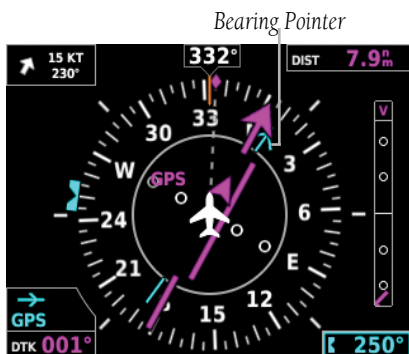
Figure 2-17 GPS Source Bearing Pointer
