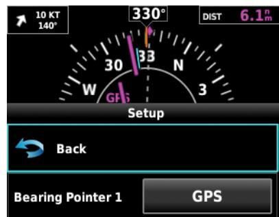
Figure 2-20 Bearing Pointer Setting
