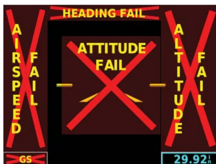
Figure 1-2 G5 PFD Page Failure Annunciations
