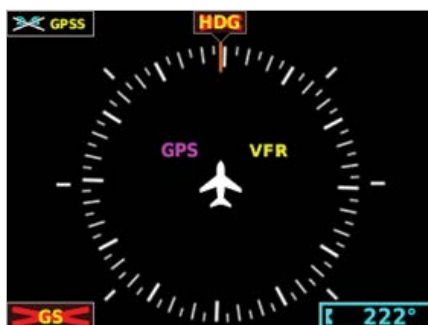
Figure 1-3 G5 HSI Page Failure Annunciations
