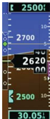
Figure 2-24 Vertical Deviation Indicator (Glideslope ILS Source) - PFD
