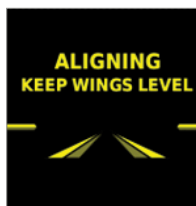
Figure 1-5 Attitude Aligning Keep Wings Level Indication
