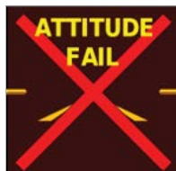
Figure 1-6 Attitude Failure Indication
