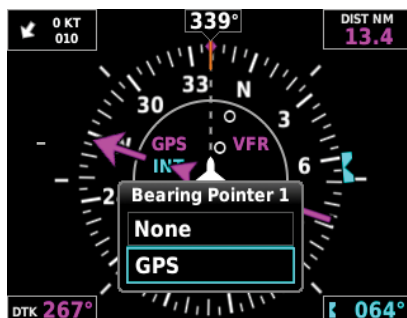
Figure 2-21 Bearing Pointer Source Options
