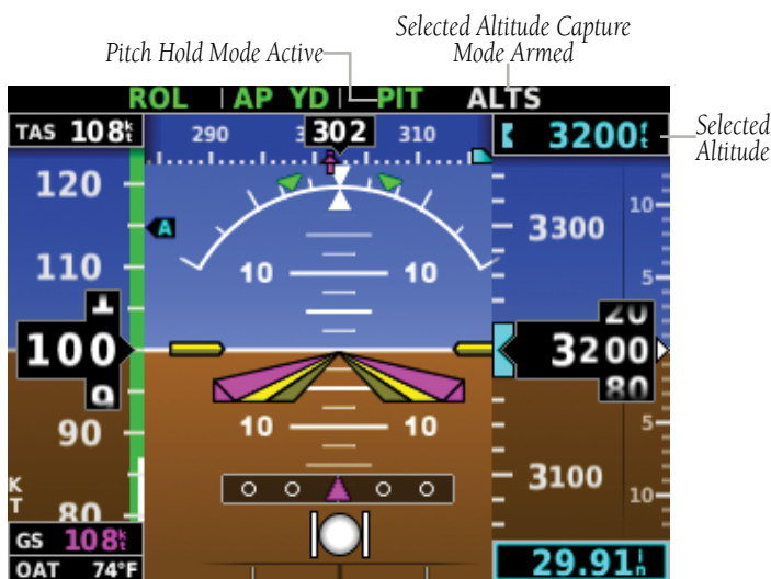
Figure 3-8 Pitch Hold & Selected Altitude Capture Modes
