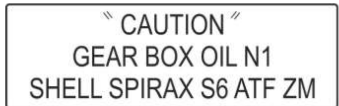
Figure 2-4 - On the inside of the oil-filler access hatch
