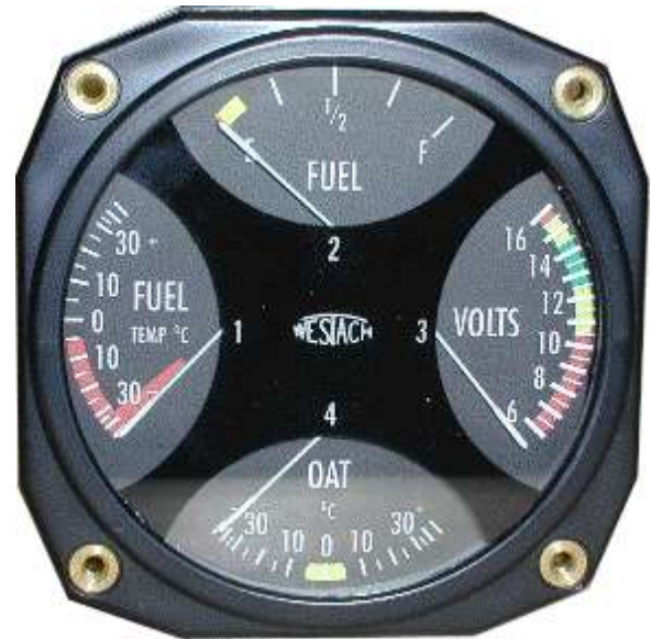
Example of Westach "quad gauge", with OAT
