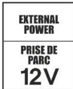
Figure 2-6 - On the access hatch of the ground power socket (if installed) on the starboard side of the aircraft.
