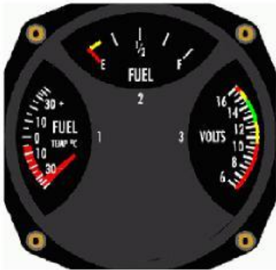
Example Of the Westach triple indicator installed on models #1 and #2
